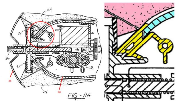
71. It is evident that Fif. 11A shows an empty gap between the medication reservoir 24 and the rigid structure 20, 26.
